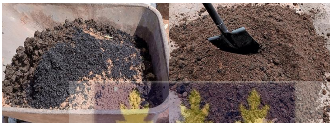
PLATE 2: Formulations from sawdust, poultry manure, rice husk biochar, top soil and clay.
