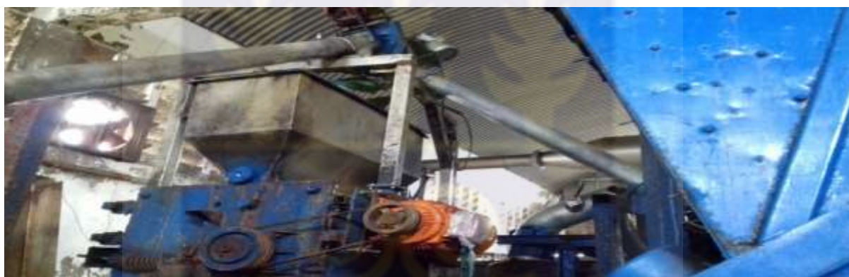
Figure 3.1. 1: A feed hopper for salt collection.
