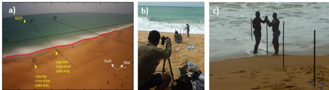
Figure 2. a) Long term camera overview. b) Poles and camera deployment to measure swash hydro-morphodynamics. c) Pole's deployment detail.
