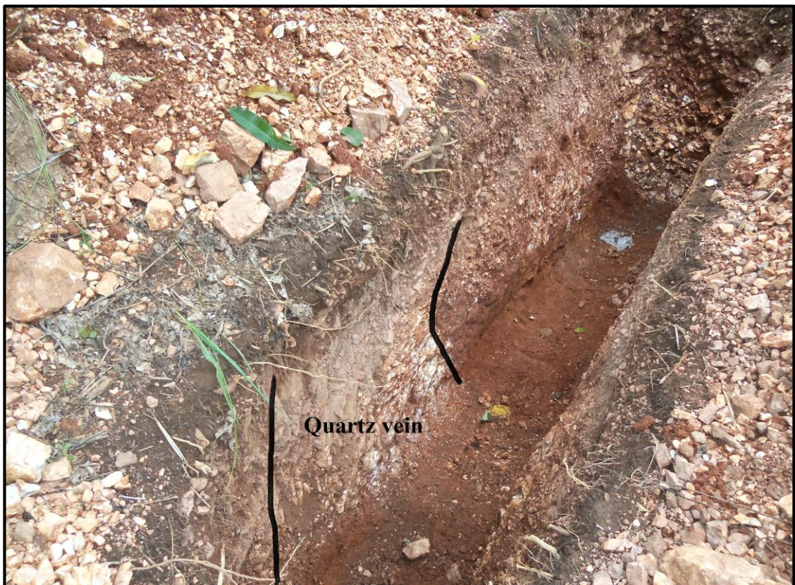
Figure 5.7: Pictorial soil profile of trench TR07- B1 shows mineralized quartz veining.
