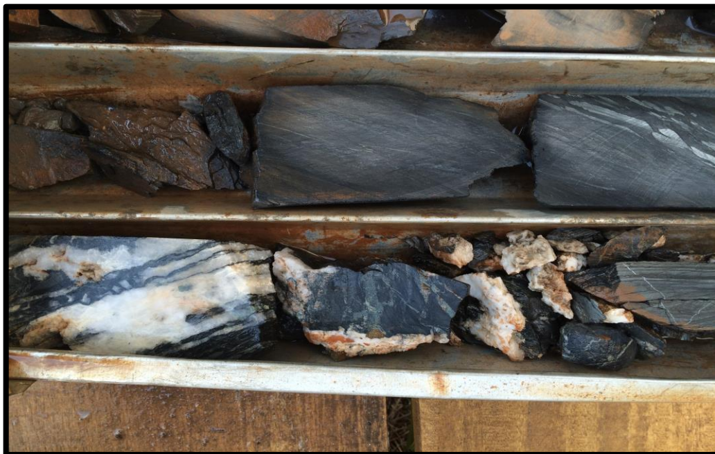
Figure 3.3: Core sample of mineralized zone of drilled hole on the study area (Kunsu property); an example of stock works style of gold mineralization.
