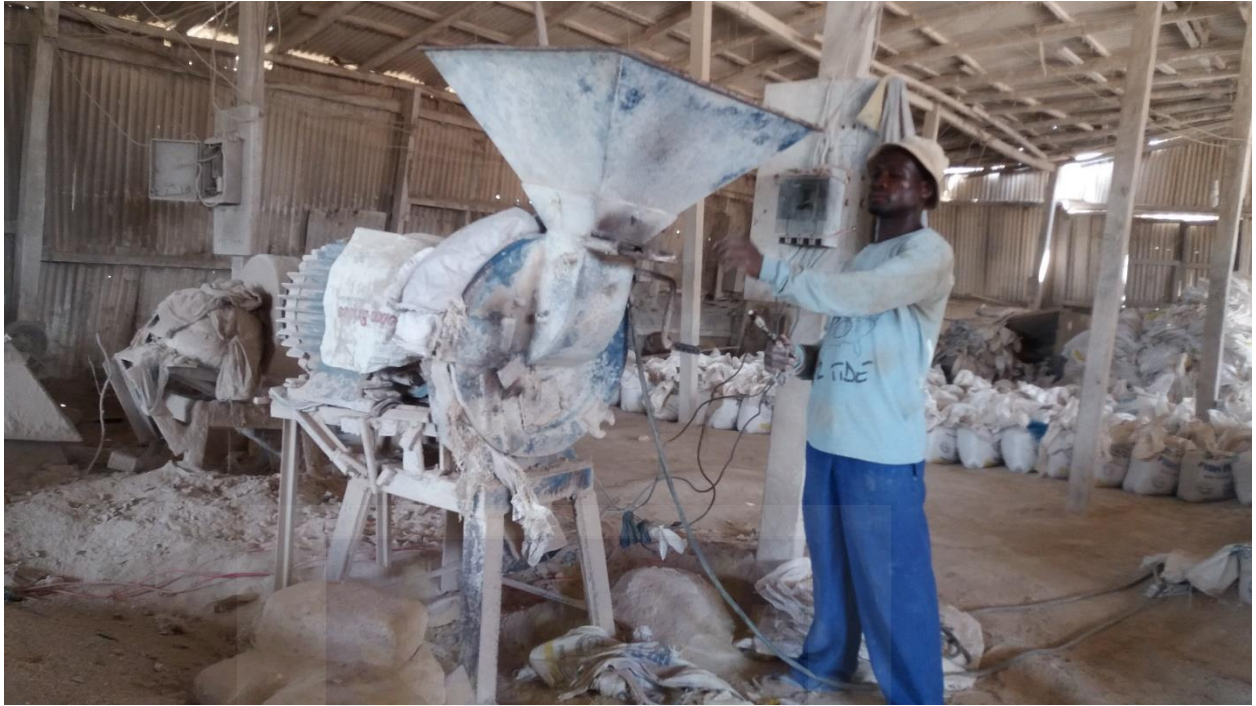
Figure 14: An oyster shell grinding machine at Akuse (Source: Beatrice Darko-Yeboah)
