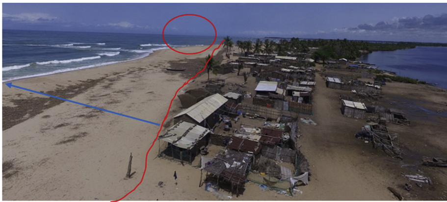
Fig. 20. Aerial view of a portion of Fuveme Showing the beach being built up. The red line shows the previous shoreline position (August 2017) and the red circle shows where the bar had developed previously while the blue arrow shows the extent of the beach that has been built (Over 80m). (Photo by Authors; April 2018). (For interpretation of the references to colour in this figure legend, the reader is referred to the Web version of this article.)
