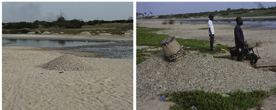
Fig. 21. Gravel mining from Nearshore at Ningo (a) Heaps of mined gravel along the beach ready for sale (b) gravel being transported via wheelbarrows to a waiting vehicle across the tidal pool in the background.
