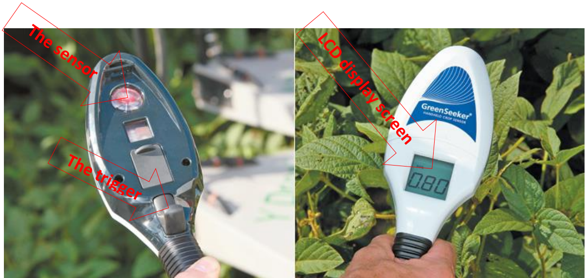
Plate 5. 2: Schematic representation of how data was captured using the Greenseeker® handheld sensor
