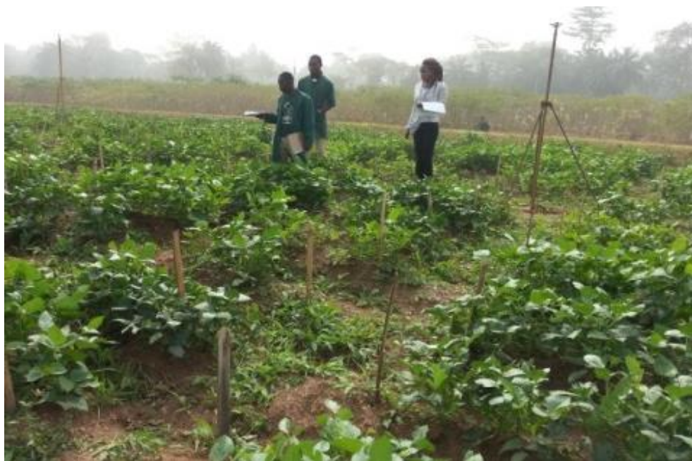
Plate 5. 3: Taking NDVI measurements on cowpea plants using greenseeker® handheld crop sensor.
