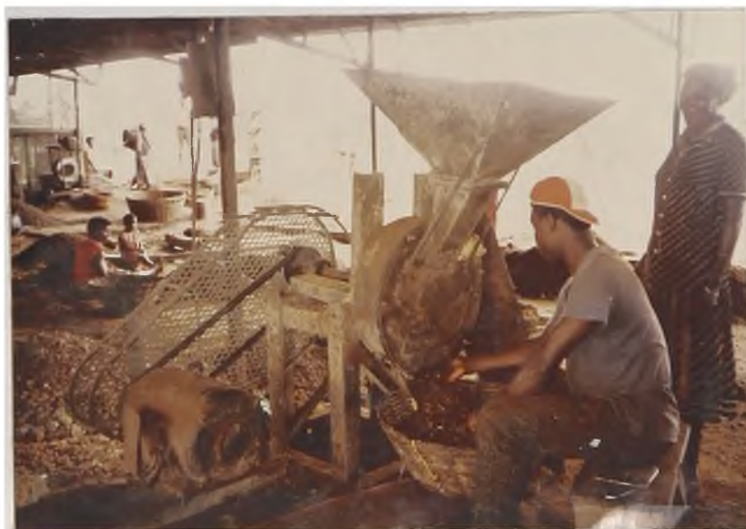
Plate 3b Motorised cracking of nuts using the nut cracker
