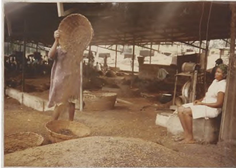
Plate 2b Winnowing of nuts/kernels. Facilitated wind dependent system. (Air blower is used to blow air over nuts/kernels as they fall)
