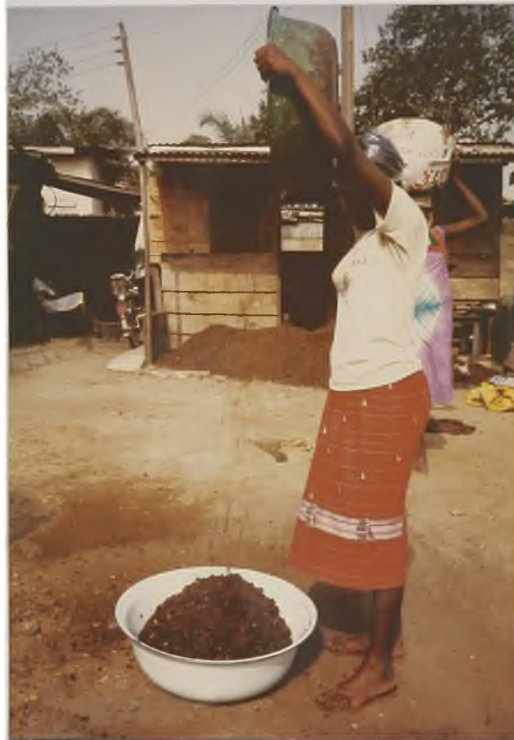
Plate 2a Winnowing of nuts/kernels The typical unaided, wind dependent system. (Nuts or cracked mass of kernels and shells are made to fall through a distance into a container along the direction of the wind. The wind blows off the lighter refuse)
