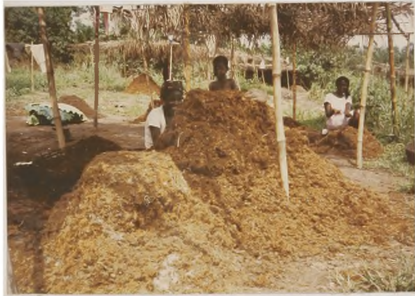
Plate 1 Separation of palm nuts from a press mass of fibre and nuts
