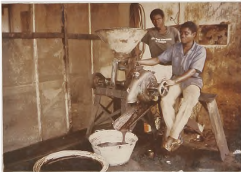
Plate 8 Milling of palm kernels using the disc attrition mill
