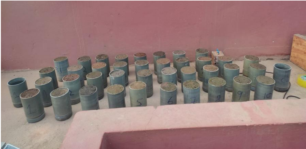
Figure 3. 4 The experimental setup for measurement of soil evaporation.
