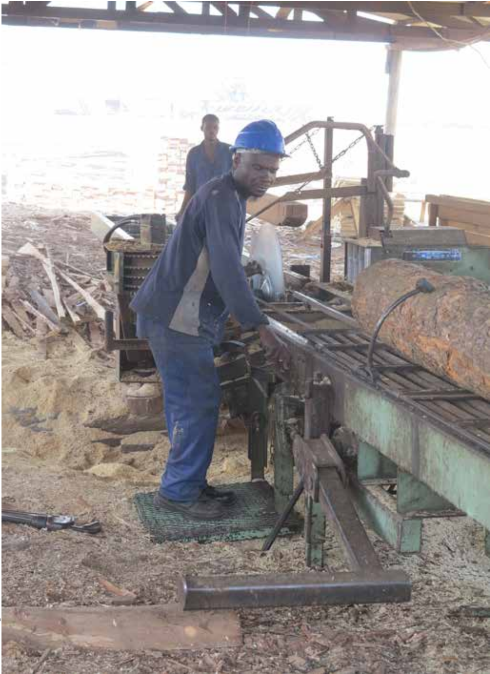
PHOTO 36 Circular saw, unguarded
