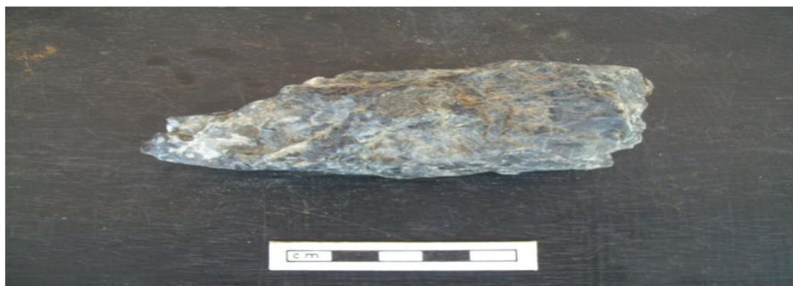
Plate 7.9. One of the few larger fragments of iron slag from the study area. Note the glass-like vitrified surface (Picture: Fritz Biveridge)
