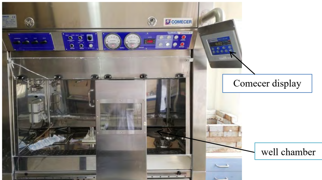
Figure 3.2: FHG LAF shielded Radiochemistry Cappa/fume hood with Comecer dose calibrator.
