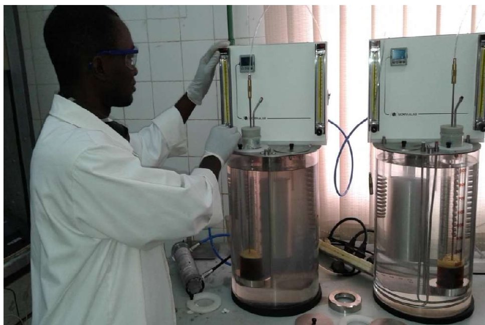
Appendix III: Aeration Control in Foam Measurement of Engine Oils Using the Foaming Bath.
