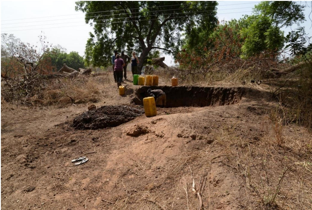
Fig. 5.12: Builders/brick makers digging into a mound for moulding bricks (Photo by D. Genequand)
