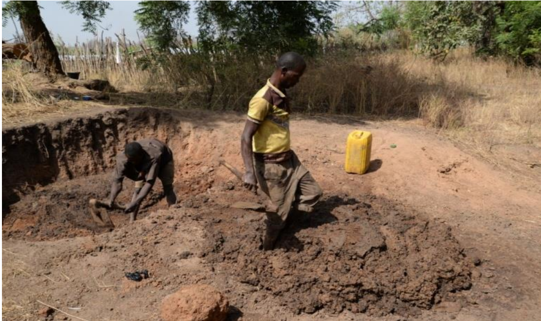
Fig. 4.7: Kneading of earth (mud) with both legs for moulding bricks (Photo by D. Genequand, 2017)
