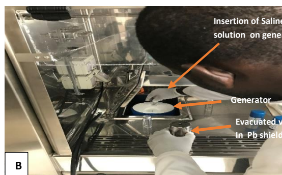
Fig 3.2B Experimental procedure of the ^{99}\text{Mo}/^{99\text{m}}\text{Tc} Generator during ^{99\text{m}}\text{Tc} eluate production
