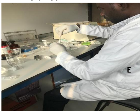
Fig.3.12E. Insertion of ITLC sections into \gamma -ray counting glass vials
