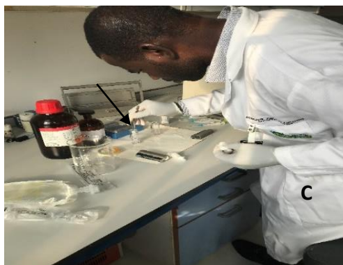
Fig.3.12C. Removal of ITLC strip from acetone chamber
