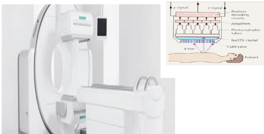
Fig. 2.5 Schematic diagram of a \gamma -camera being used for \gamma -rays detection emitted by a radiotracer distributed in a patient
