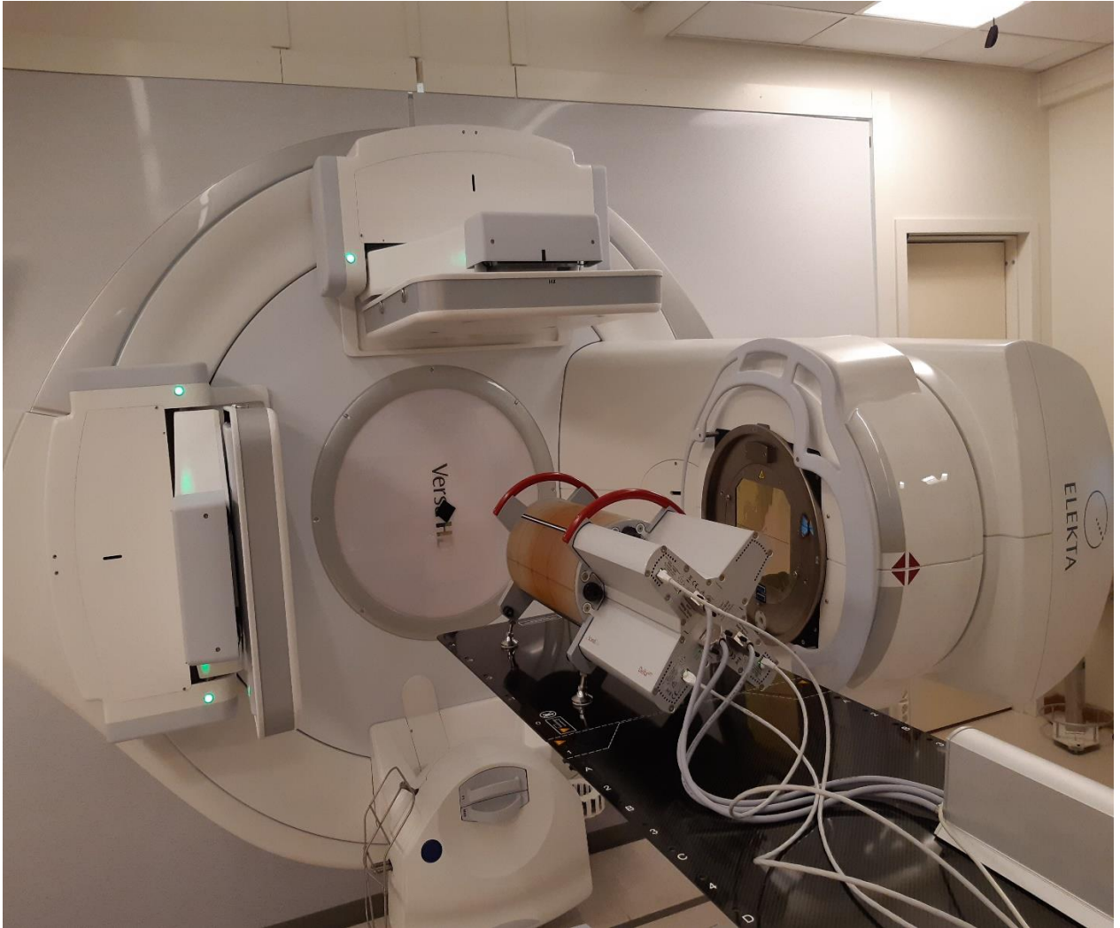
Figure 3.4: An image showing the setup for determining the factor of the day for both 6 MV and FFF beam at 90^\circ .
