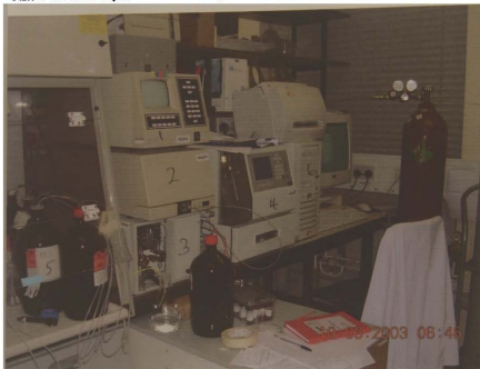
(1) Controller (2) Photodiode array detector (3) Pump (4) Autosampler (5) solvents (6) Computer (7) Carrier gas
