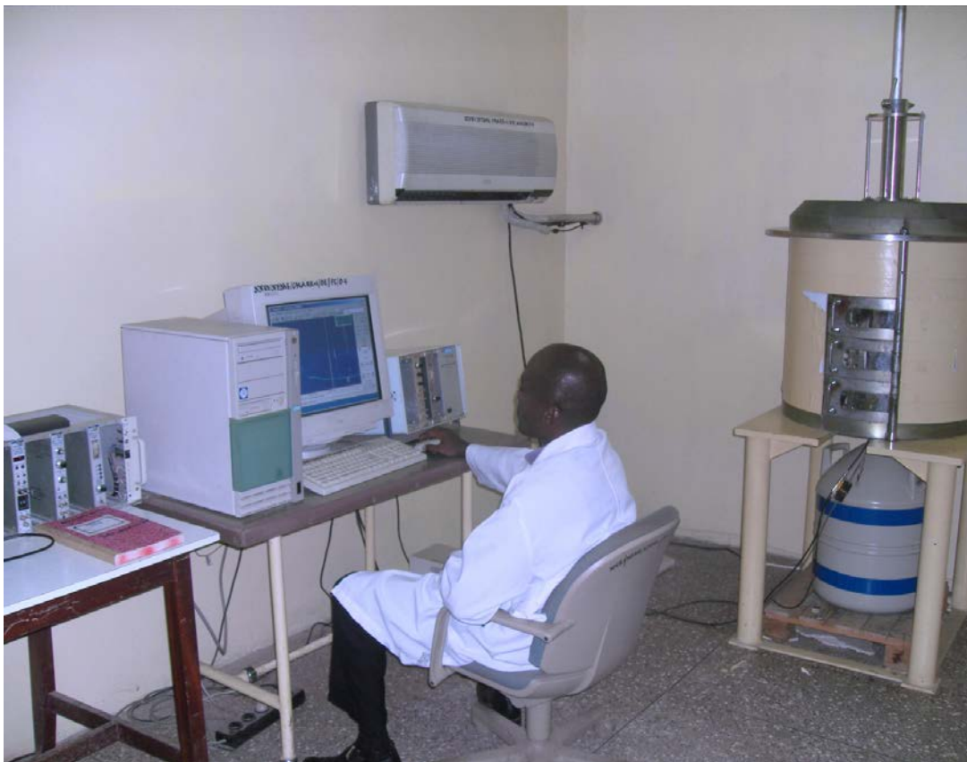
Plate 4.1: The High Pure Germanium Detector assembly used for analysis of the samples of beach sand at the Ghana Research Reactor – 1.
