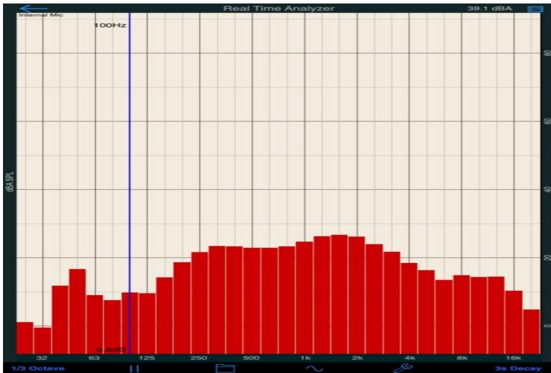
Fig. 4.2: Sample of the spectral characteristics of ambient noise in the quiet office (39.1dBA)
