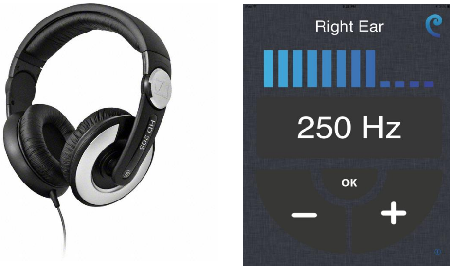
Fig. 1.1: Sennheiser HDA 205 headphone (left) and ACEScreening application software interface (right).
