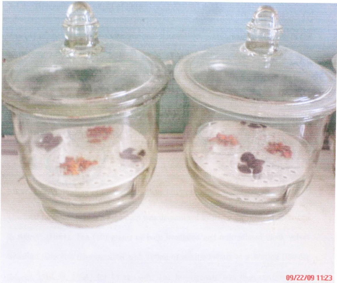
Plate 3: Photograph showing the arrangement of the black velvet tamarind inside glass desiccators (Note: The glycerol: water mixtures simulating the prescribed ERH's were poured into the bottom of the container) (X 1/100)
