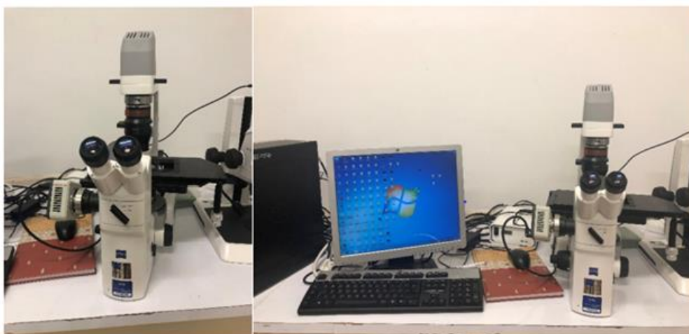
Figure 12. Setup of ZEISS Axio Vert A1 Inverted Phase Fluorescence Microscope.
