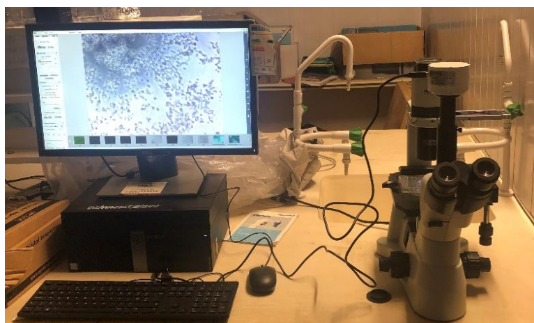
Figure 11. Setup of Optika Microscope (Italy) equipped with an Optikam B9 Digital Camera.
