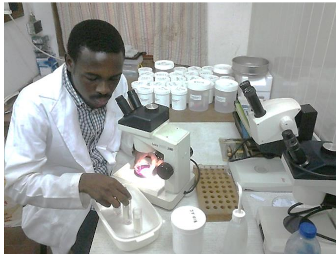
Plate 3.3 - Macrobenthic identification using the stereomicroscope.
