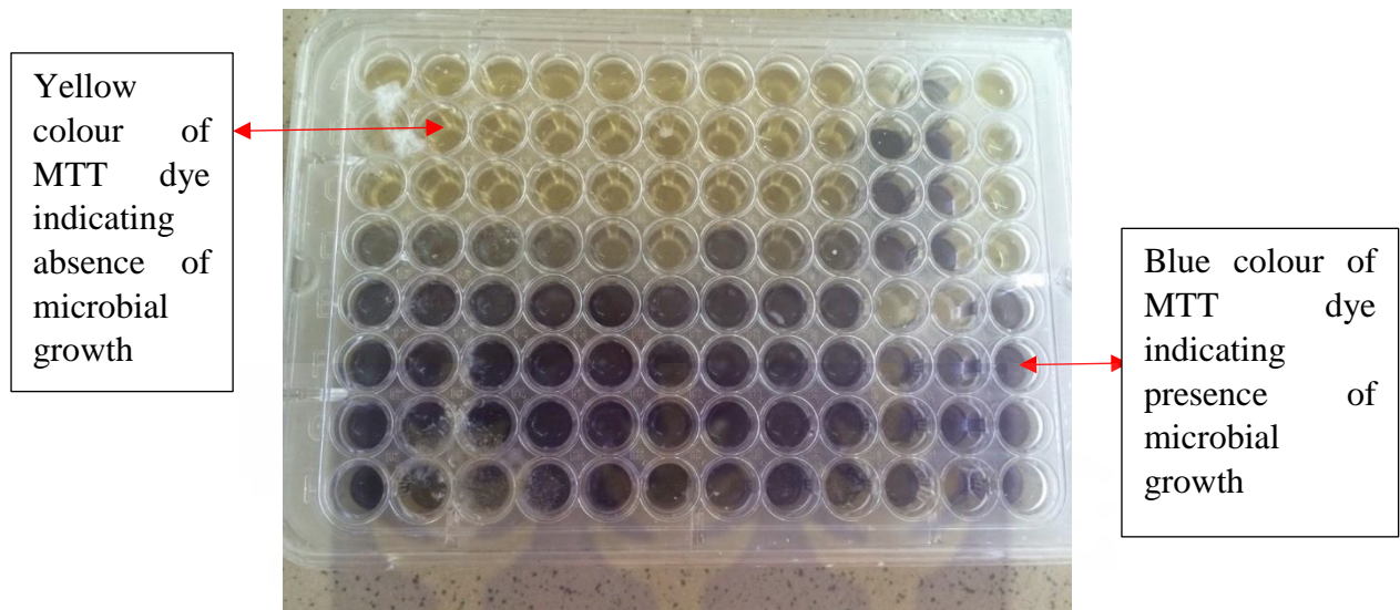
Fig 2.5: A 96-well micro-titre plate showing growth and no-growth for MIC determination (Talaro, 2002)
