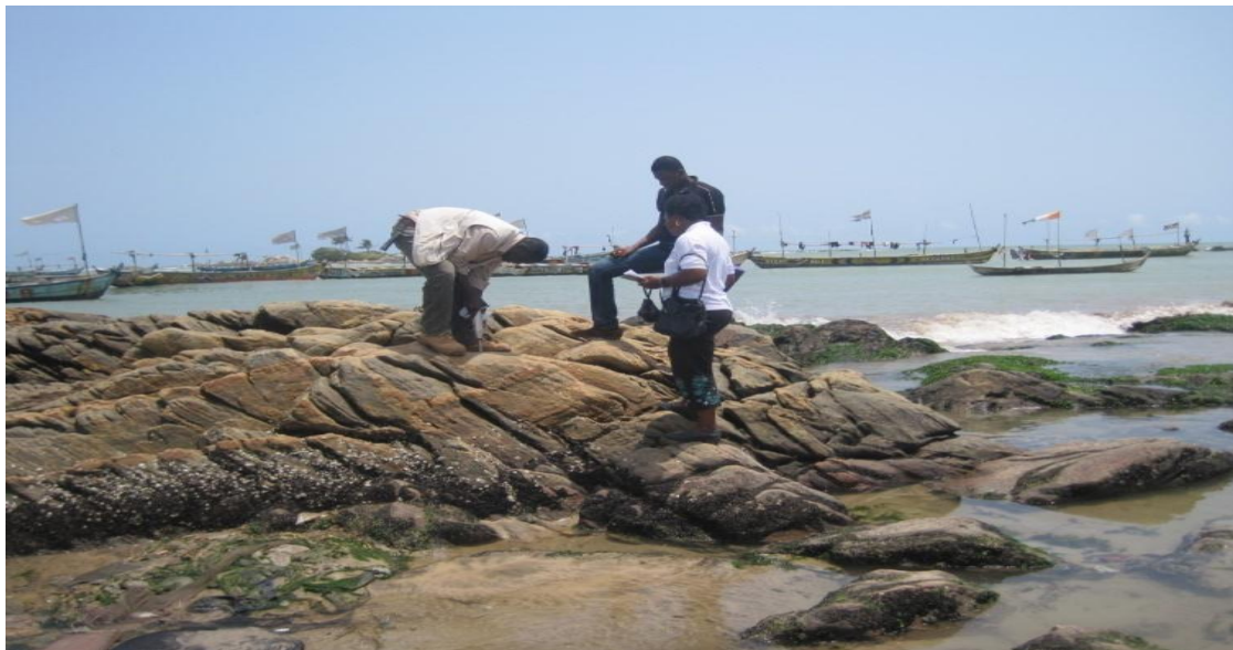
Figure 9: Photograph showing Measurement of Rebound Value at Abuesi
