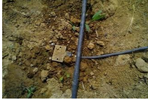
Figure 3.3. TDR probes with extended cable
