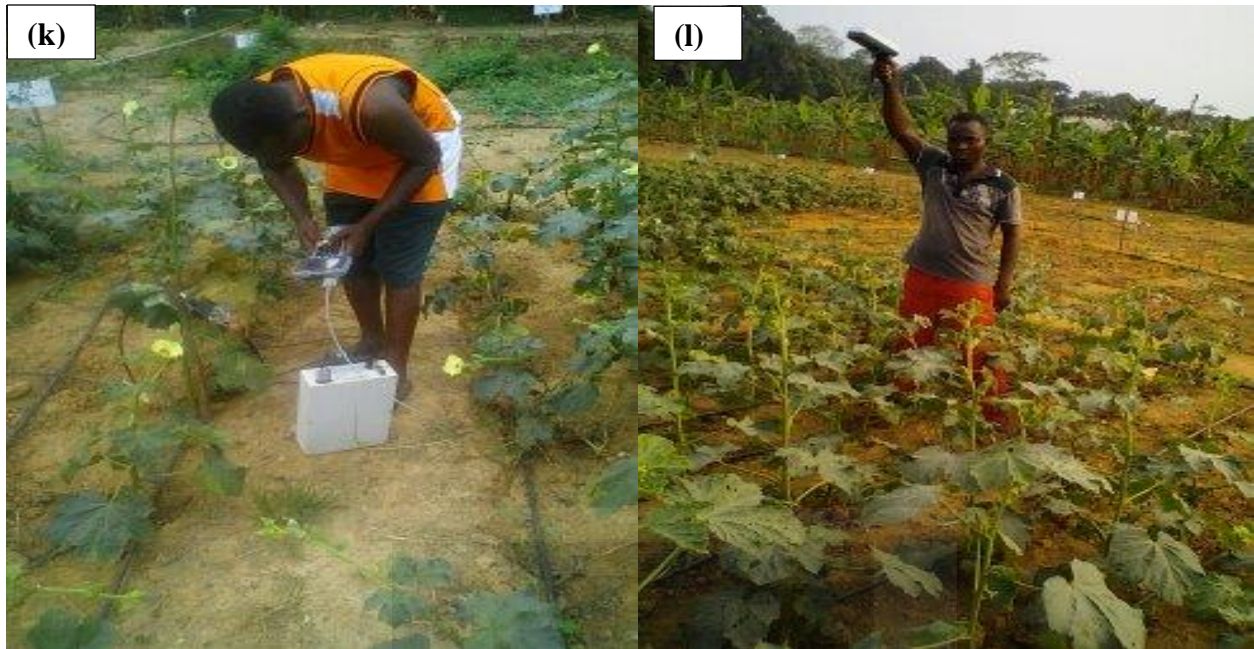
Figure E7. (k) Measuring SWC with TDR and (l) Measuring okra vegetation index (NDVI) with RapidSCAN CS-45
