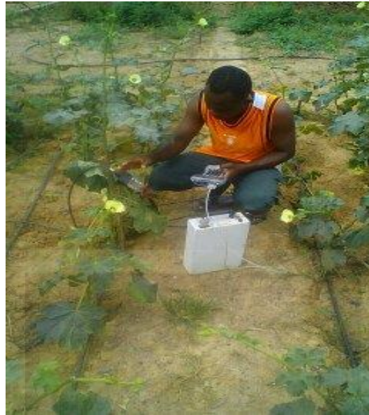
Figure 3.4. Measuring SWC with TDR
