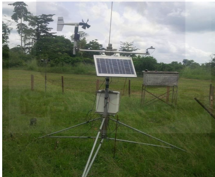
Figure 3.6. Automatic weather station at the research centre
