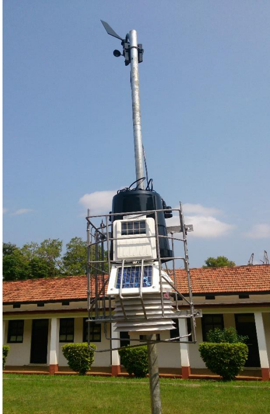
Figure 4.12: Complete ISS setup communicating with console
