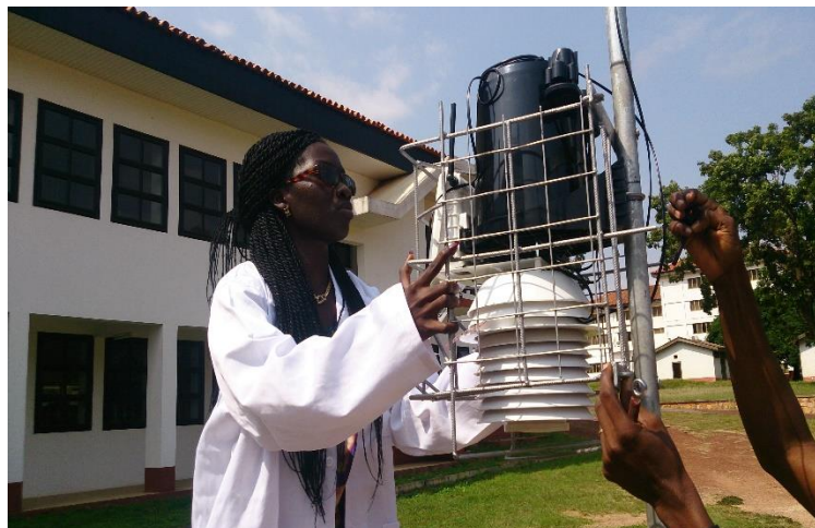
Figure 4.11: Positioning the protective cage around the weather station at the Physics Department, University of Ghana
