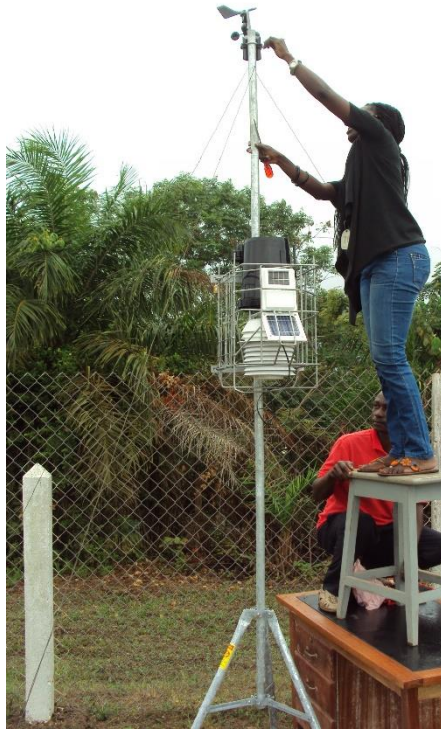
Figure 4.13: Setting up the Davis Vantage Pro 2 Weather Station at the Axim site
