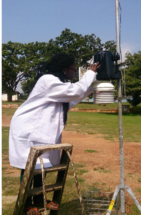
Figure 4.10: Setting the Transmitter ID for communication between the ISS and the console
