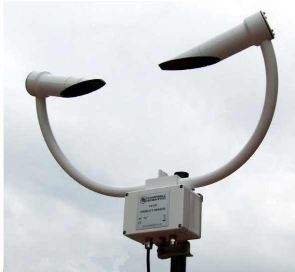
Figure 4.5: Campbell Scientific CS120 Visibility Sensor
