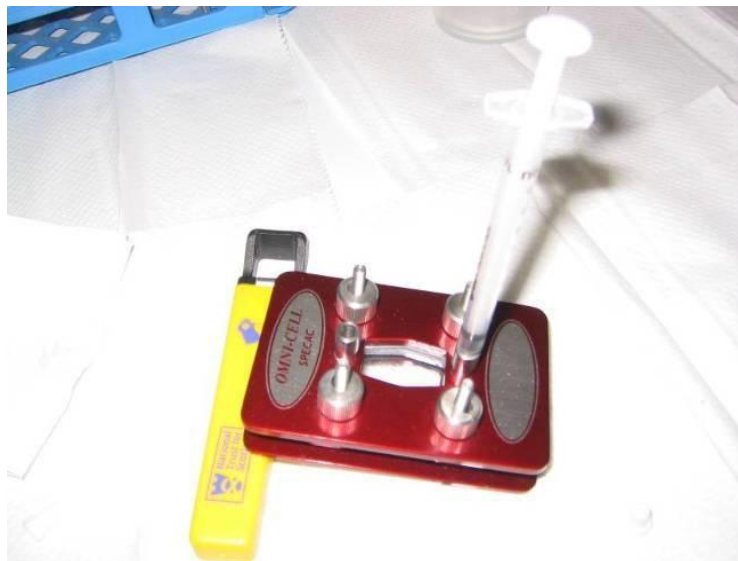
Fig 3.4: FTIR cell with a 1 ml syringe in the filling port (IAEA, 2010).
