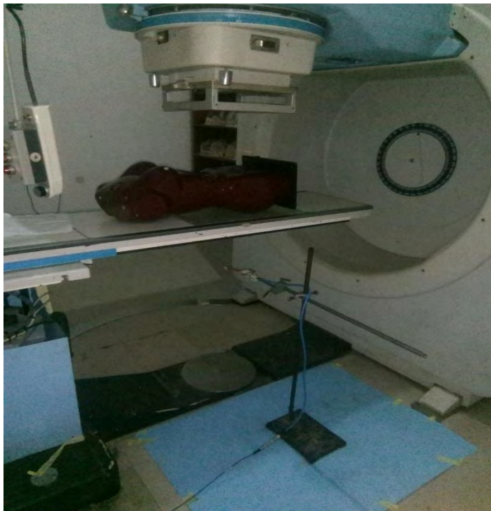
Figure 3. 10: set-up for ionization chamber exit dose measurements under anthropomorphic phantom
