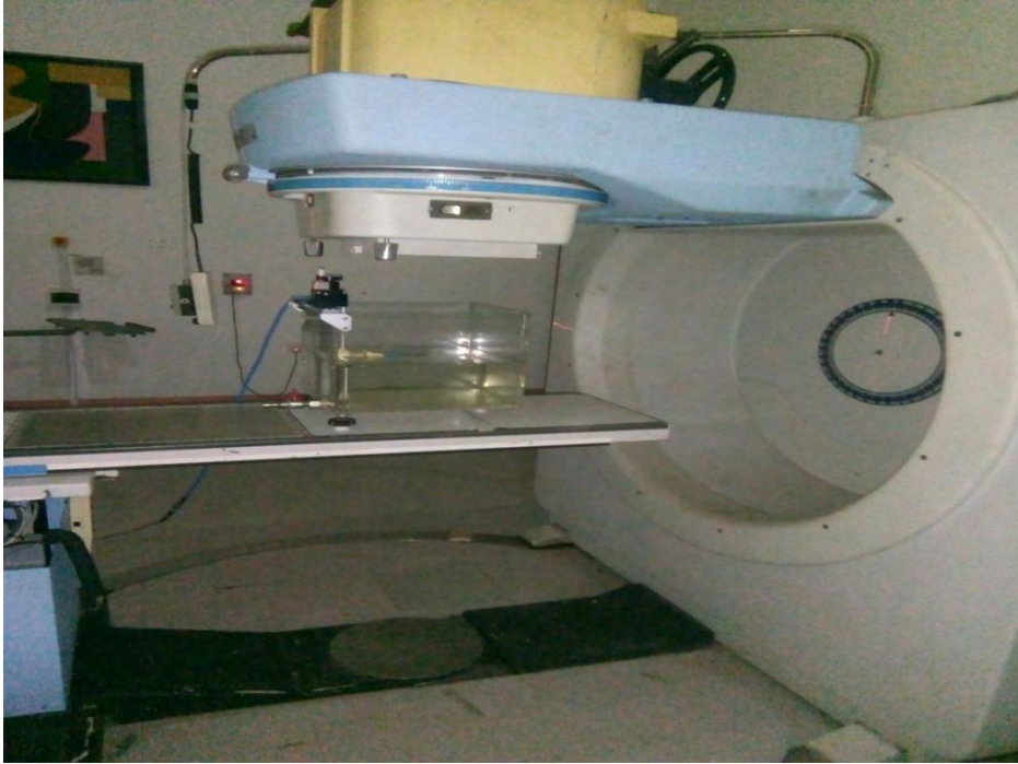
Figure 3. 9: Setup for couch transmission factor determination
