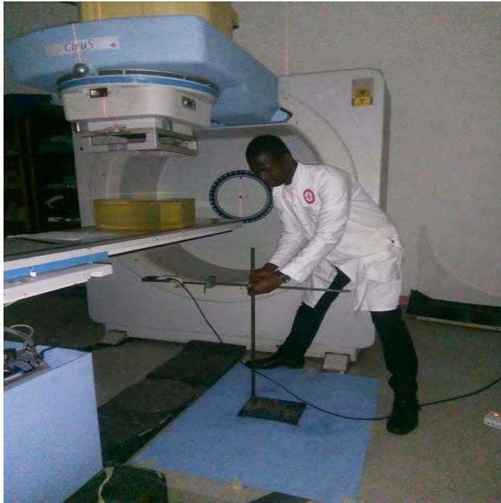
Figure 3. 11: Set-up for barracuda exit dose measurements under Perspex slab phantom
