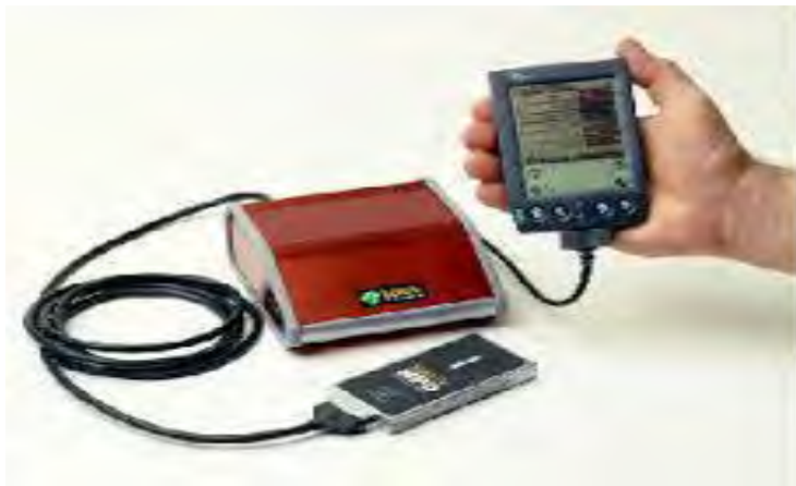
Figure 3. 6: The Barracuda system; cabinet, multi-purpose detector and a palm-held computer
