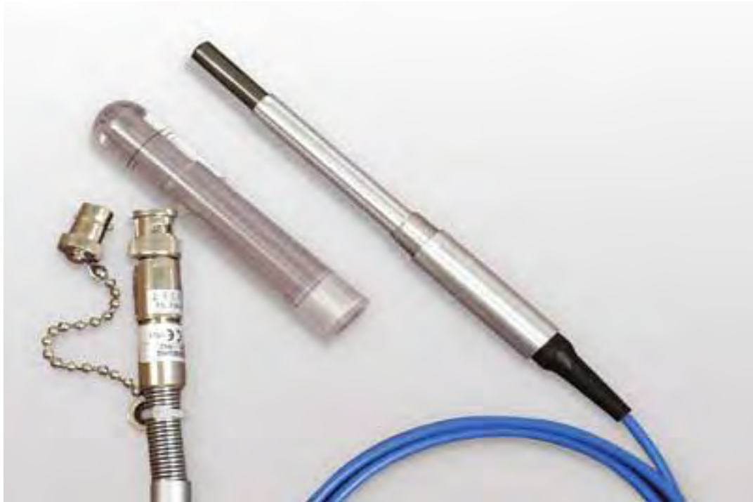
Figure 3. 2: Farmer type ionization chamber (PTW Freiburg, Germany)
