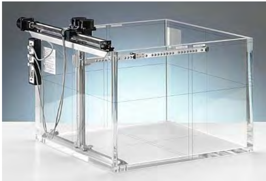
Figure 3. 4: A 30 \times 30 \times 30 \text{ cm}^3 water phantom
