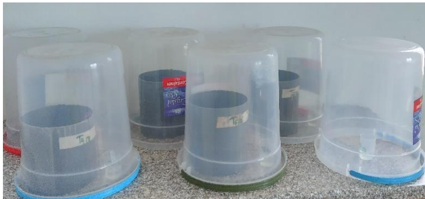
Figure 3. 2 Layout of laboratory experiment showing chambers for trapping emitted carbon dioxide
