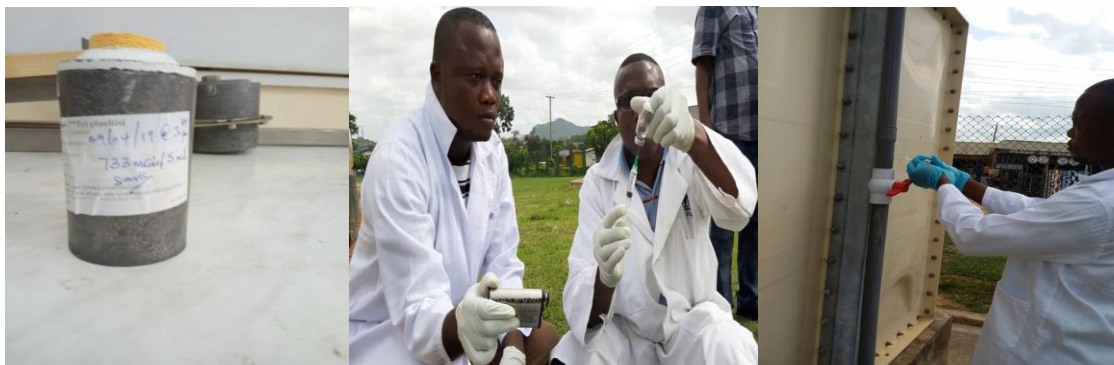
Figure 3.3 Tracer in a lead shield, Tracer loading and Tracer injection syringe
