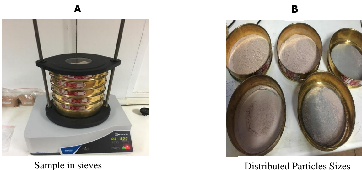
Figure 8: Process for Determining the Particle Size Distribution of Composite Flour Samples
