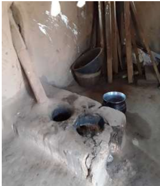
Plates 4. 2: Cracked ICS
