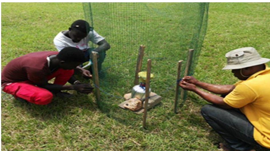
Figure 3. 6: A fabricated rainfall collector mounted at St Patrick Catholic Church in Half Assini.
