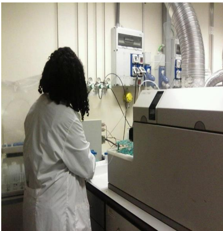
Figure 3. 9: ICP-MS used for the measurement of trace elements in the water samples.
