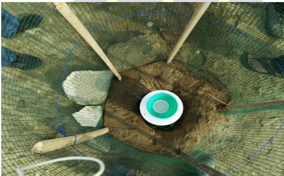
Figure 3. 5: IAEA donated rain collector mounted at Edjah Villa in Esiama
