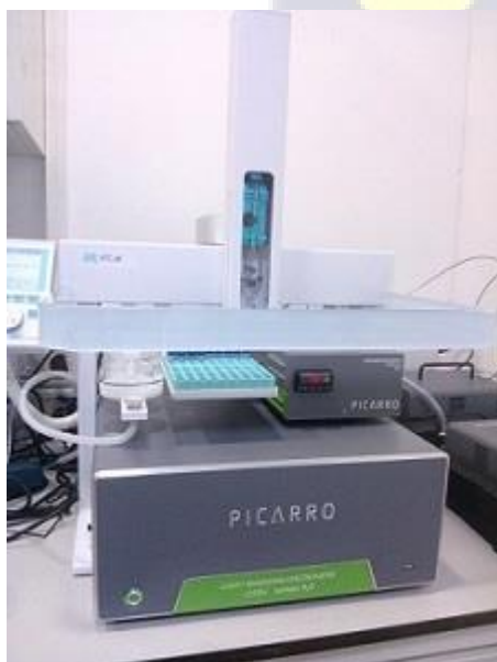
Figure 3. 11: Picarro L2130-i used for the measurement of \delta^{18}\text{O} and \delta^2\text{H} in the water samples with its auto sampler.
