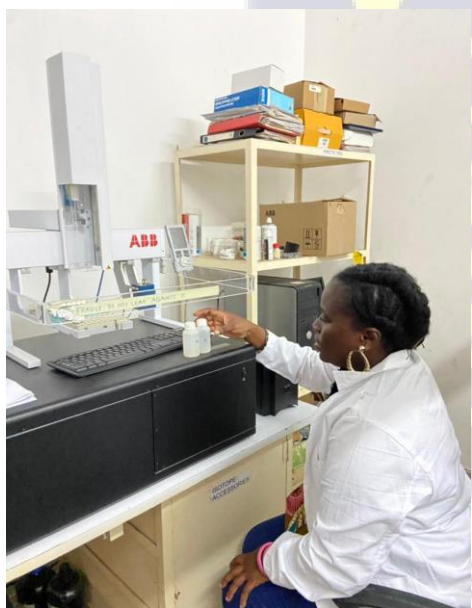
Figure 3. 10: Isotopic composition analysis ( \delta^2\text{H} and \delta^{18}\text{O} ) of the water samples using Los Gatos DLT-100 Liquid-water Stable Isotope Analyzer.
