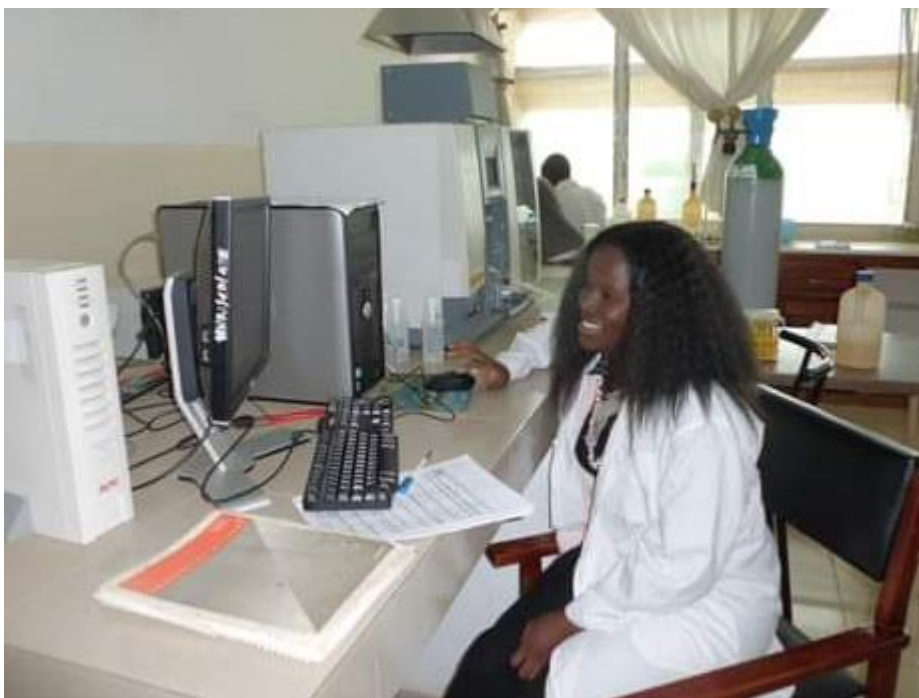
Figure 3.8: Fast Sequential Atomic absorption spectrometer (VARIAN, AA 250 FS, Australia) used for the analysis of trace elements.
