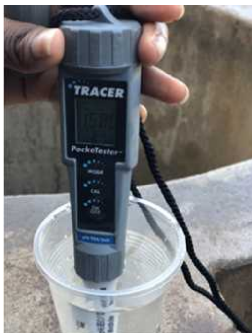
Fig. 3.5 LaMotte PockeTester used for measurement of physical parameters
