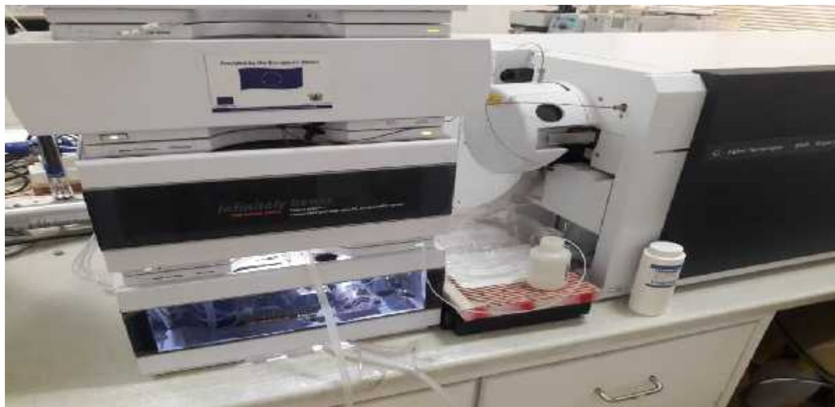
Fig. 3.9: Agilent 1290 Infinity series LC-MS/MS facility in the Pesticide Residue Laboratory of Ghana Standard Authority used for identification and quantification of Glyphosate residues
