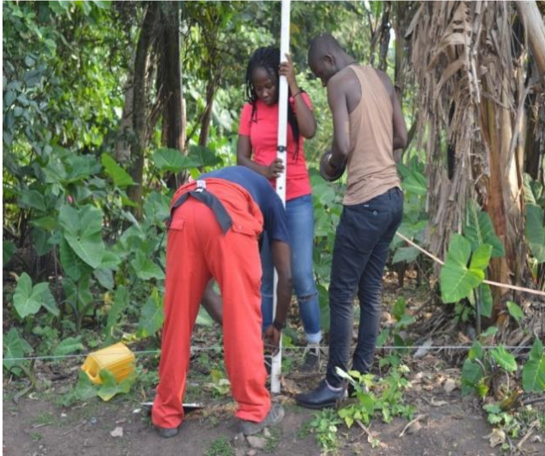
Figure 4.17. Mapping the surface of the Obosomase site using a total station and a stadia rod. (Photo
