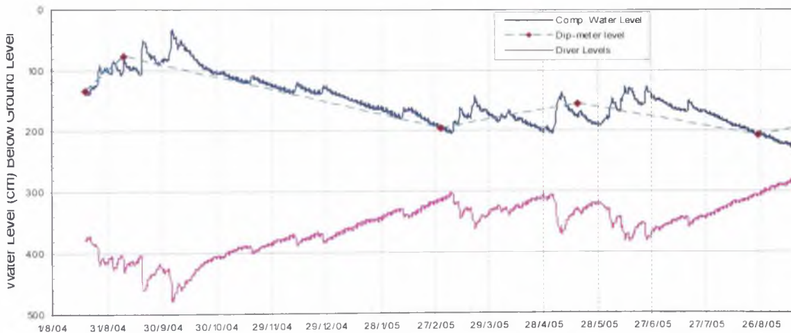
Fig 8.6 Groundwater level – time graph at Adwumoko monitoring stations (Water Research Institute 2006)
