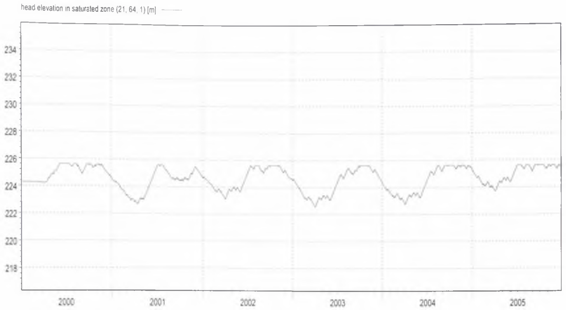
Fig 8.13 Groundwater head elevation in the Granite for the entire simulation period (2000 – 2005)
