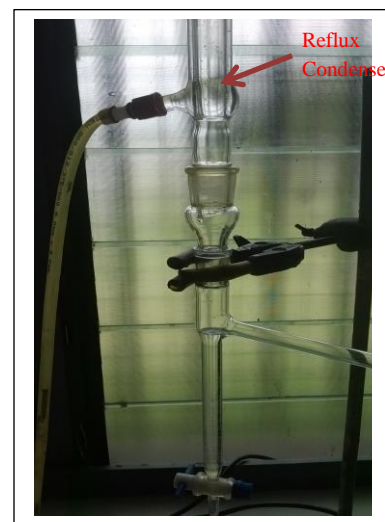
Fig 3.6c Reflux condenser at point of insertion with glass trap
