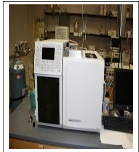
Fig 3.14f GC-MS instrument Varian CP-3800
