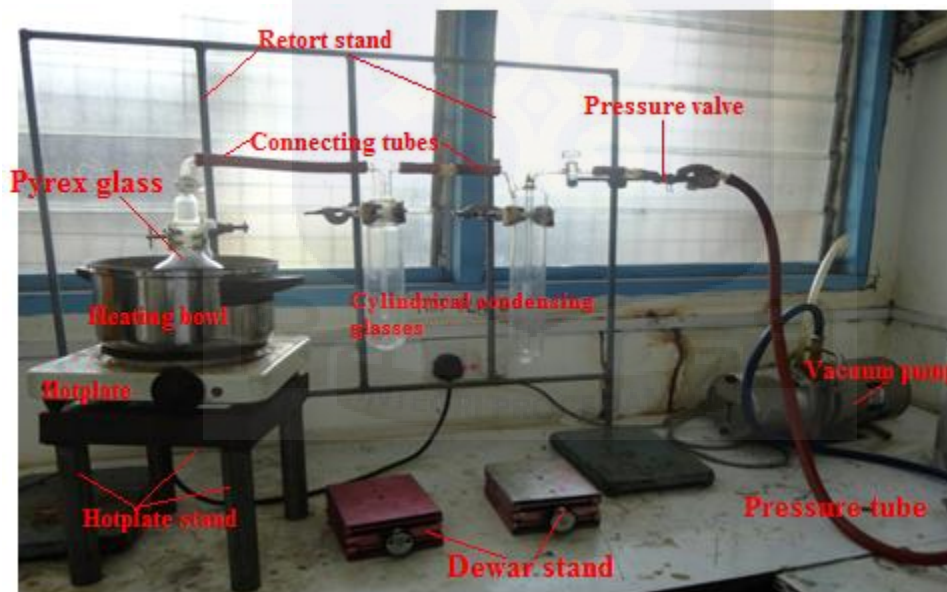
Fig 3.4: Soil moisture extraction system without moisture trap and showing system being degasing.
