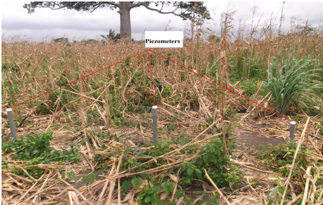
Fig. 3.3 Installed piezometers in the study area
