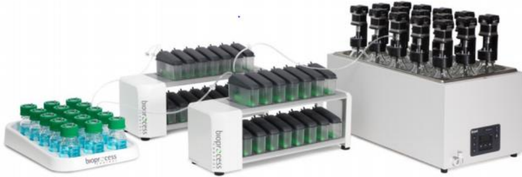
Fig. 3.2. AMPTS II comprising of temperature-controlled water-bath, reactors with overhead stirrers, alkali solutions and flow meter cells.
