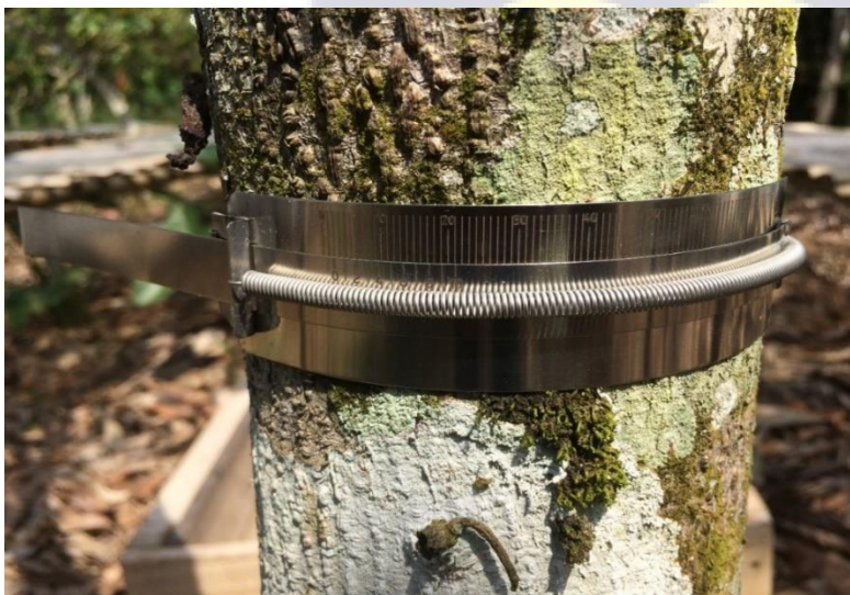
Plate 3.2.5 Dendrometer Bands Wrapped Around the Circumference of a Cocoa Tree
