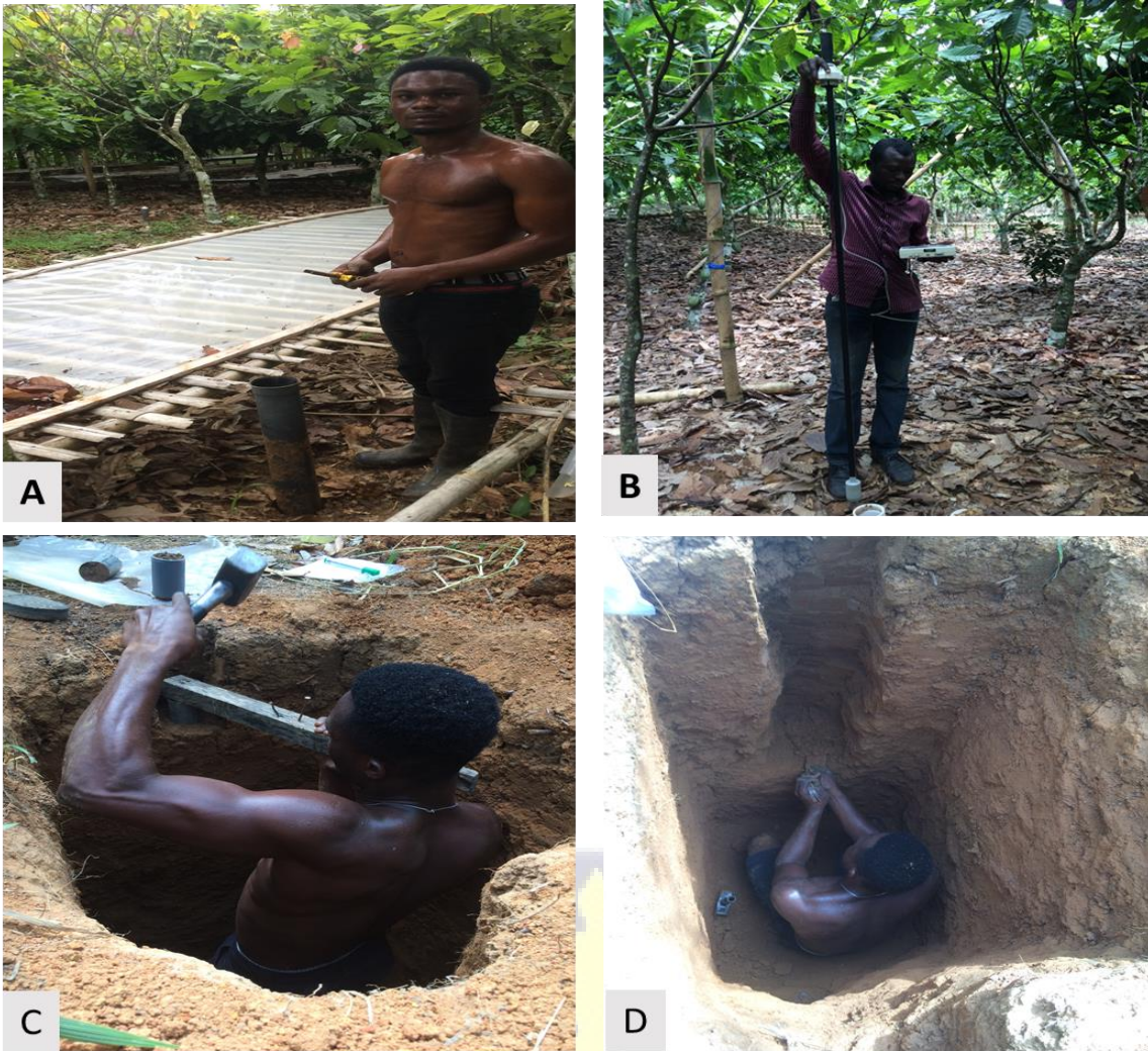
Plate 3.2.2 Monitoring Soil Moisture Content Using Diviner Soil Moisture Sensor (A and B) and a Core Sampler (C and D)
