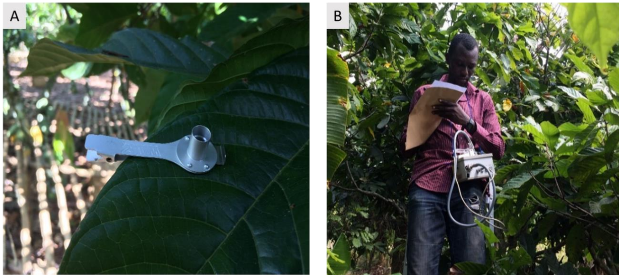
Plate 3.2.4 Measuring Chlorophyll Fluorescence Using Mini-PAM. A – Cocoa leaf with light exclusion clips; B – Taking readings from mini-PAM after measurement of chlorophyll fluorescence.
