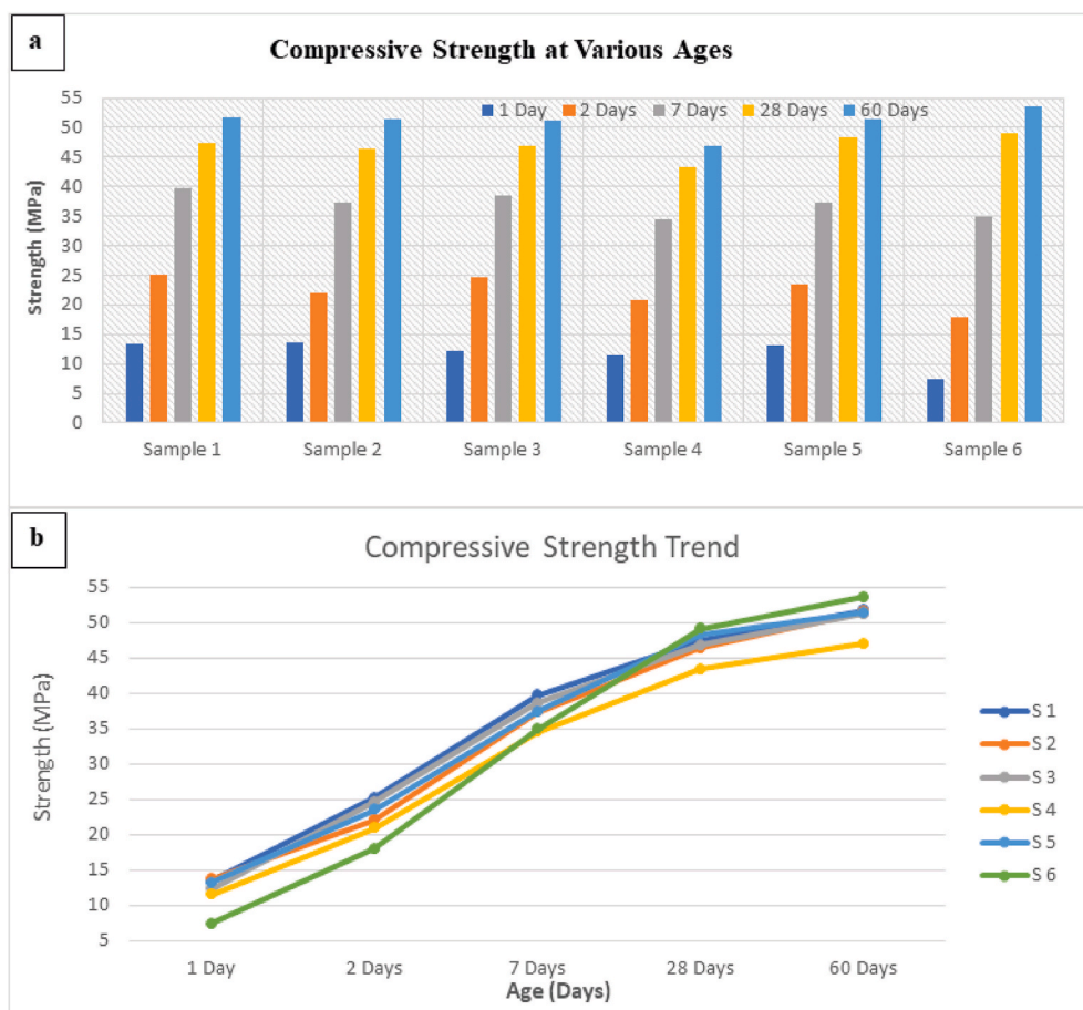
Fig. 5. (a) Compressive strength increases in days (b) Compressive strength showing increasing trend in days.
