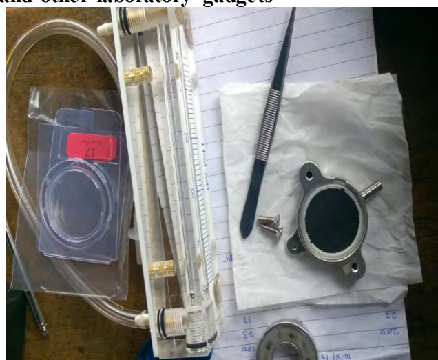
A filter taken out in the research mini lab after a 24hr deployment in the field
