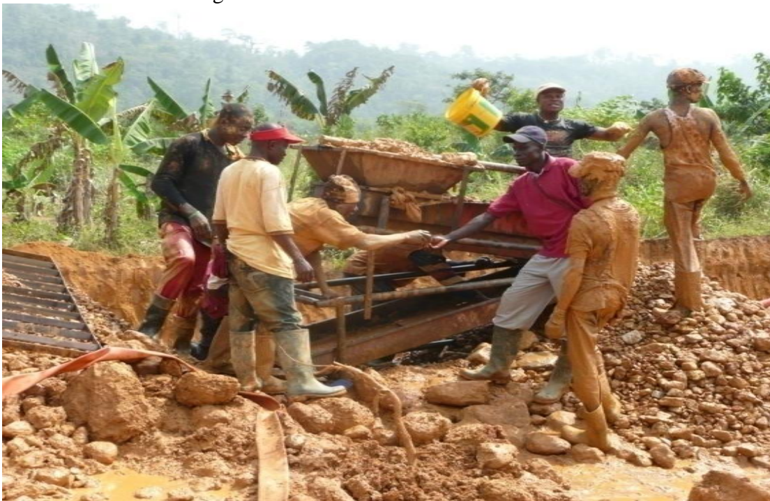
Plate 2: Miners Washing Sand with a Sluice Box for Gold
