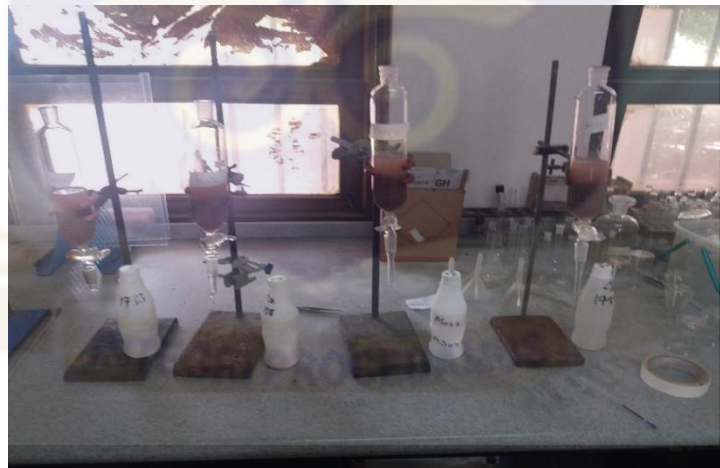
Fig 3.15: Iron Samples in volumetric Separation funnels
