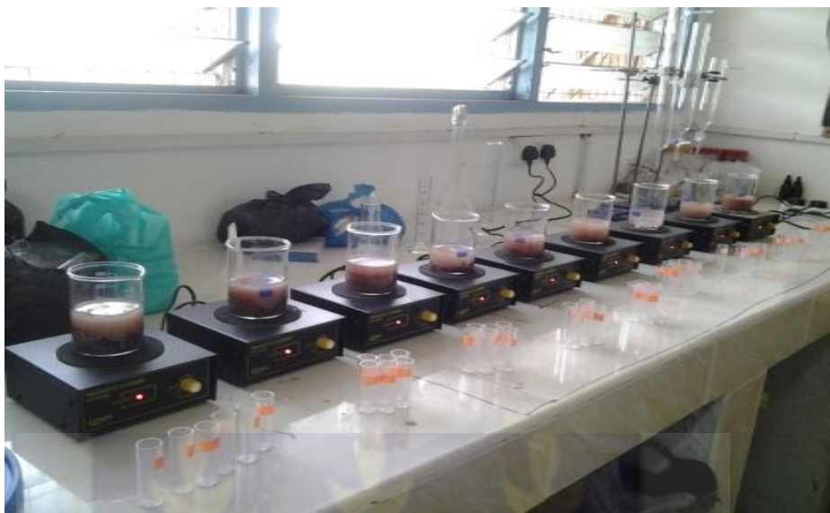
Fig 3.8: Batch setup showing mixtures agitated by magnetic stirrer on orbital shakers
