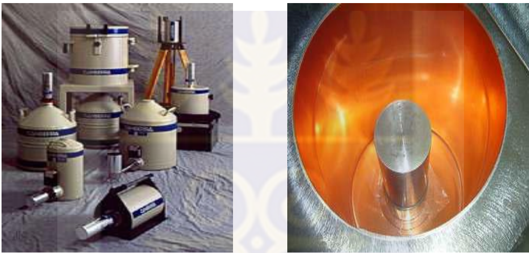
Fig 2.3: Examples of \gamma -ray detectors
