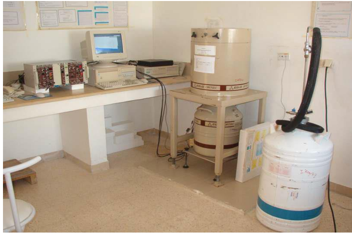
Fig 2.4: Typical example of a gamma spectrometer setup
