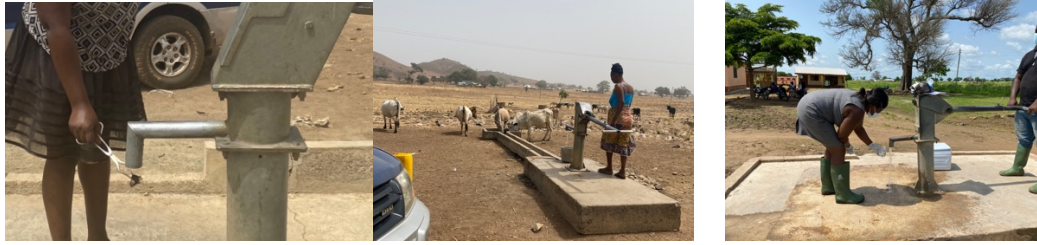
Flaming and sampling from borehole
