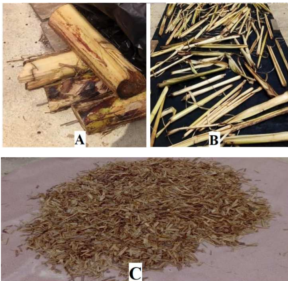
Plate 3.2 Plantain pseudostem preparation in stages: A- Freshly harvested plantain pseudostems B- Freshly chopped plantain pseudostems C- Dried shredded plantain pseudostems
