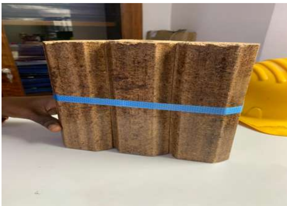
Figure 4.2 Bricks to replace firewood and to be used in the clean stove above
