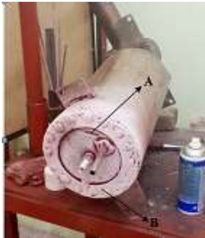
Figure 4.9: Result of the dye Penetrant test.
