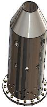
Figure 3.17: The Inner Liner Assembly Design
