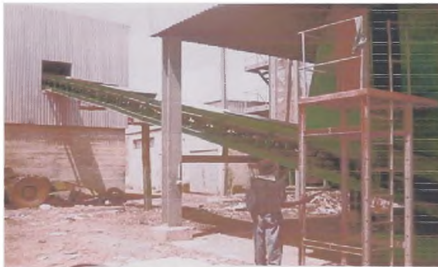
Plate 6: Conveyor belt carries compost down into the green automated separator at Teshie site.
