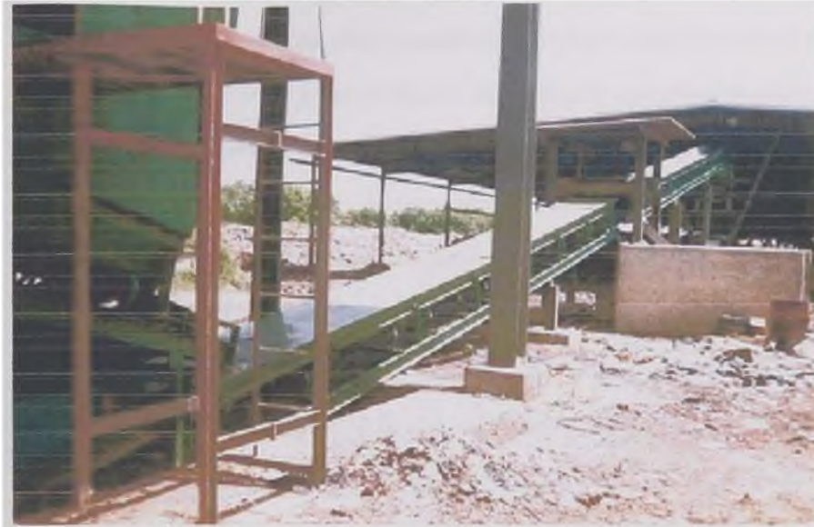
Plate 7: Separated compost is carried up the conveyor belt from the green separating device into the shed where compost is stored and ready for bagging.
