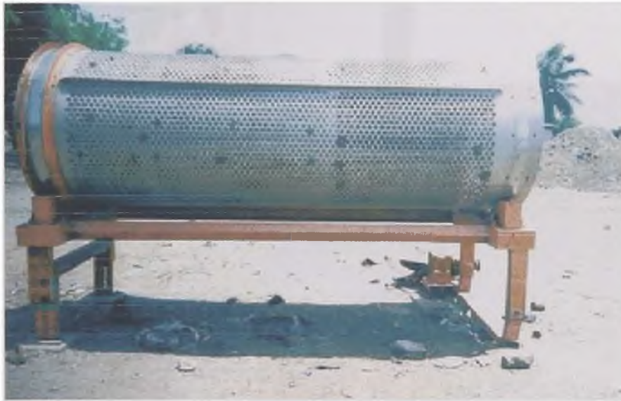
Plate 5: Manually operated sieve used for separation of contaminants from compost at the Asiedu-Keteke site.
