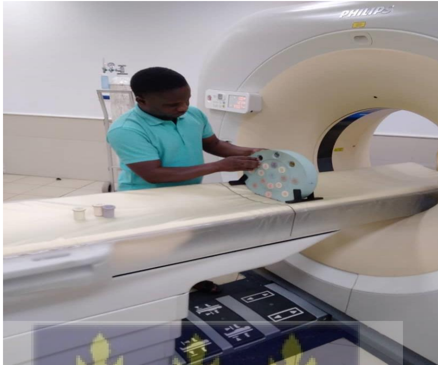
Figure 3. 11: A set-up of the ED phantom for CT scan during the study.
